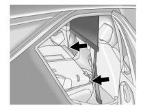
Mount the cargo net to the rear seat tethers located on the front of the bottom cushions.
